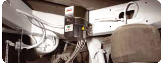
Lincoln's Quickclub automated lubrication system eliminates the need to manually lubricate under the trailer
