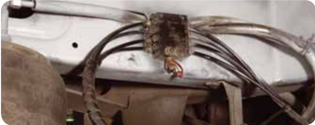
Lincoln's single point kit brings together all trailer lubrication points into one – saving valuable maintenance time
