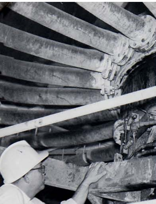
IMC lubrication engineer, at left, inspects SL-1 injectors on rotating filter head.
